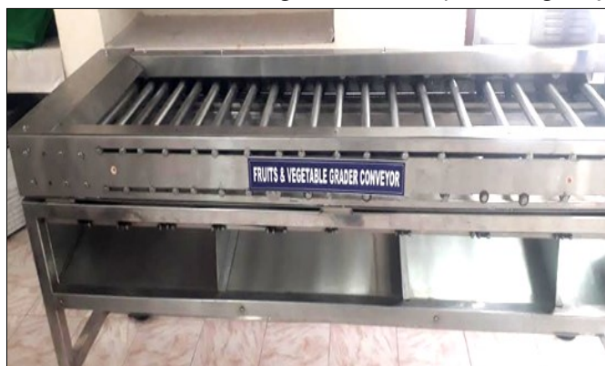
Fig. 12. Grader for fruits and vegetables.
