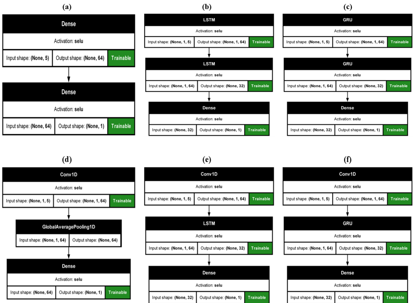
Fig. 2. Model Architectures: (a) Artificial Neural Network (ANN); (b) Long-Short Term Memory (LSTM); (c) Gated Recurrent Unit (GRU); (d) Convolutional Neural Network(Conv1D); (e) Conv1D-LSTM; (f) Conv1D-GRU.
