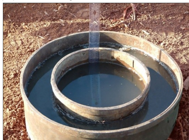
Fig. 1. Double ring infiltrometer.
