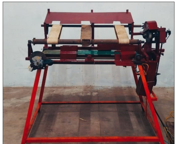
Fig. 6. Prototype of the battery-operated automated sugarcane bud sett cutting machine.
