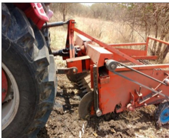
Fig. 5. Tractor PTO-operated turmeric digger-cum-separator in field (38).
