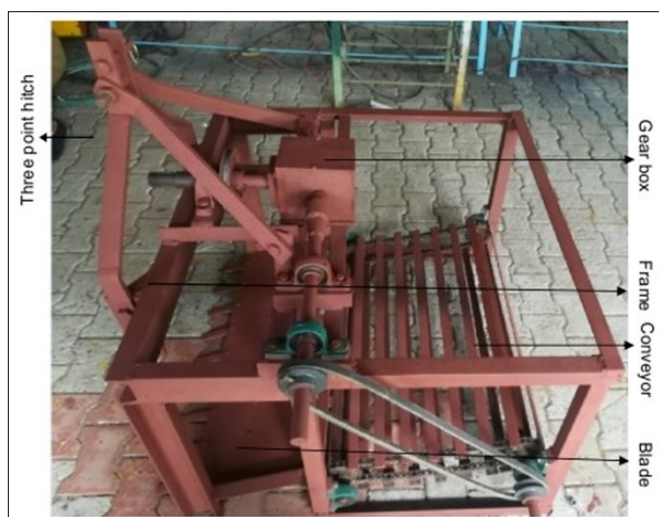
Fig. 6. Mini tractor operated turmeric harvester (55).
