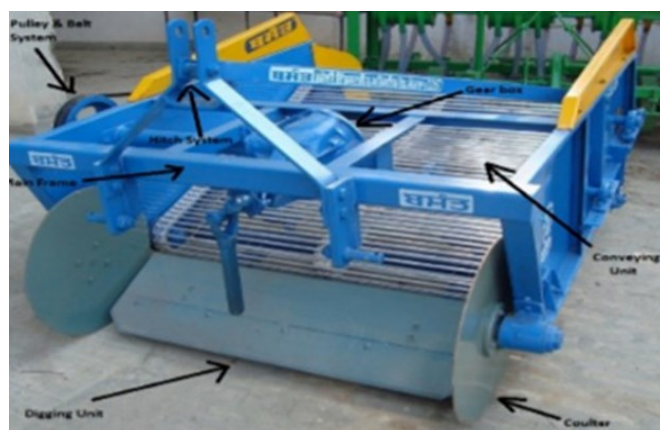
Fig. 7. Tractor drawn root crop harvester for potato and ginger crop (58).
