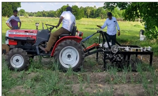
Fig. 20. Field evaluation of mini-tractor operated onion detopper and digger.
