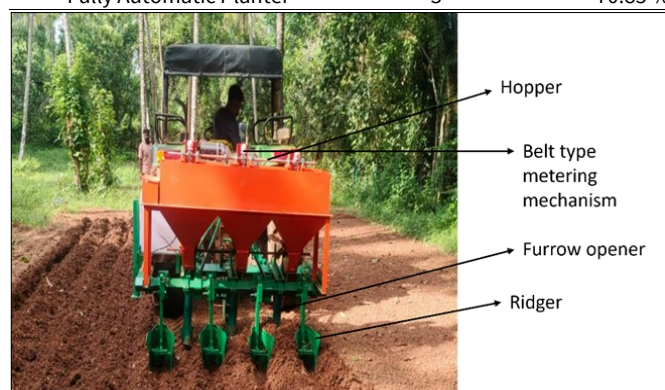
Fig. 9. Fully automatic turmeric planter (39).
