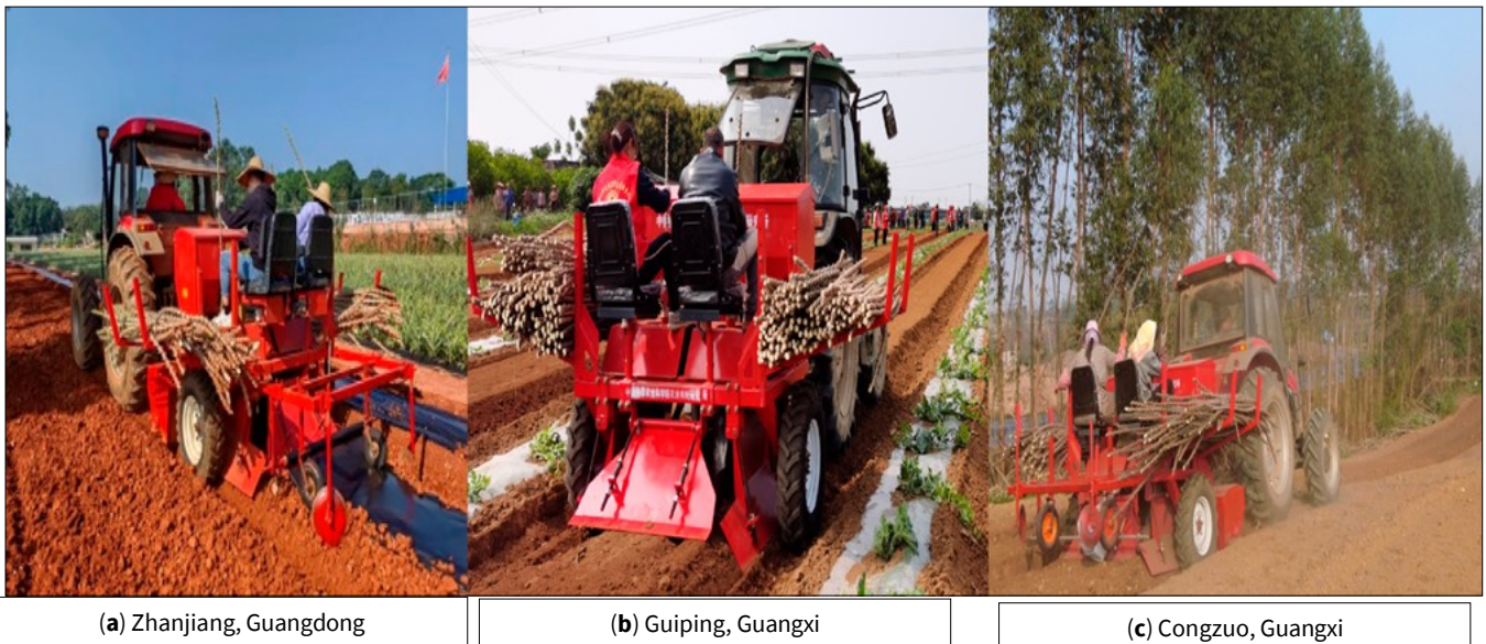
Fig. 9. 2CM-2B cassava intercropping machine in action during partial field operations (21).
