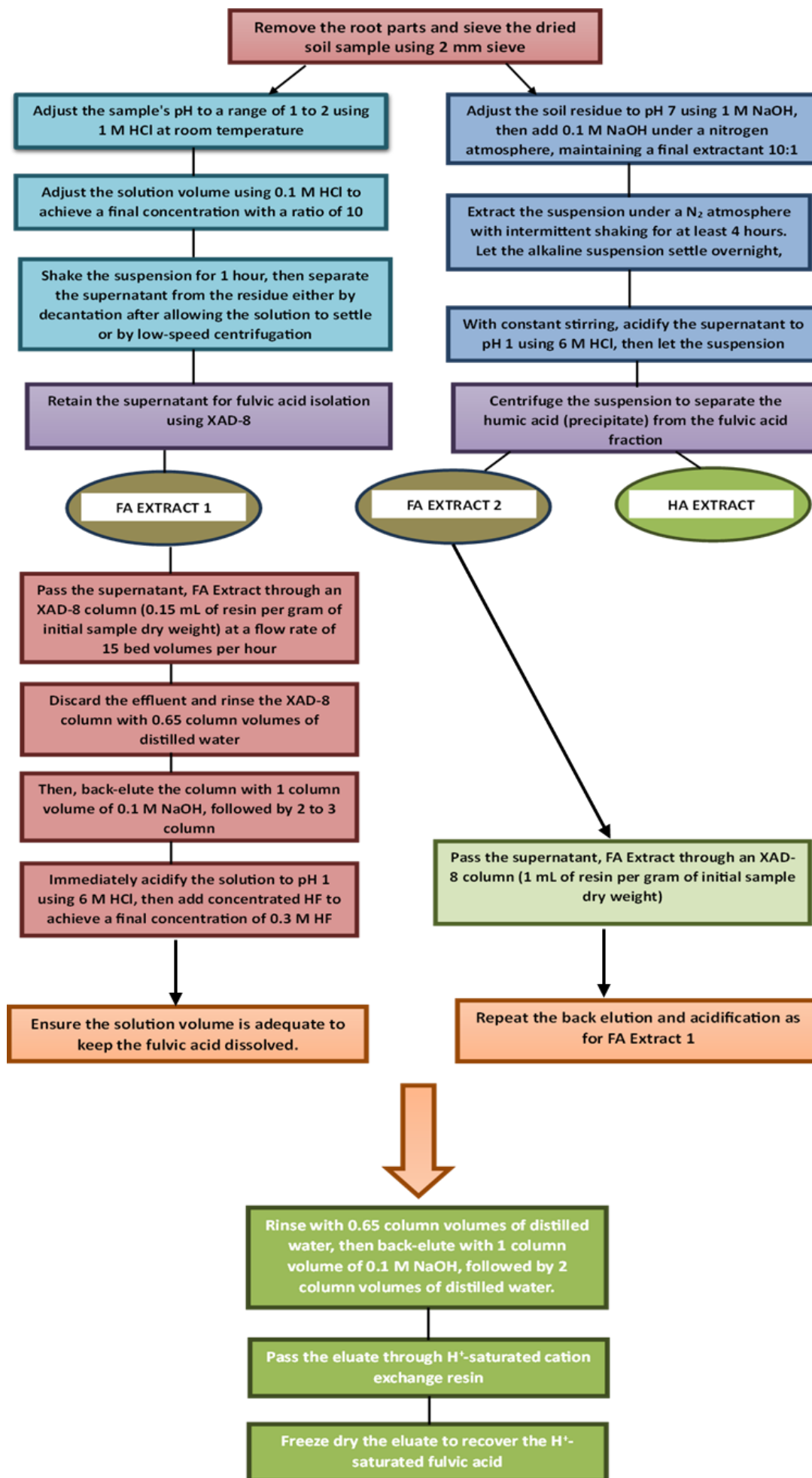
Fig. 3. Procedure for extraction of FA from soil samples given by IHSS.
