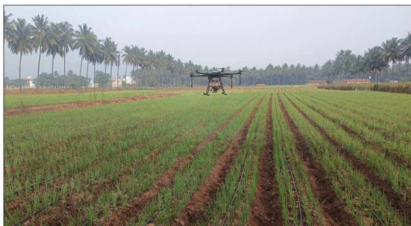
Fig. 2. Spraying of agriculture input using drone in onion crop.
