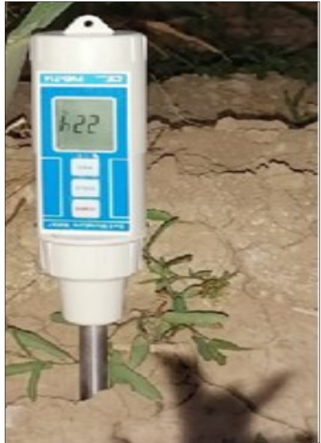
Fig. 2. Moisture measuring device in the field.
