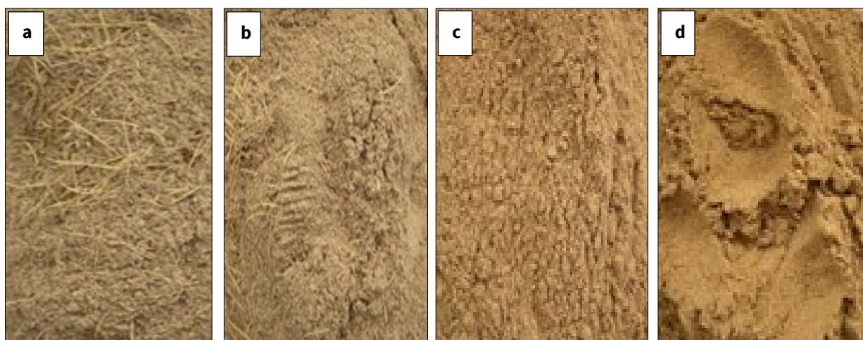
Fig. 7. Rhizome powder of H. cochinchinensis . (a. unsieved powder, moisture content 10.1 %; b. powder passed through 0.450 mm sieve; c. powder passed through 0.300 mm sieve; d. powder passed through 0.150 mm sieve).
