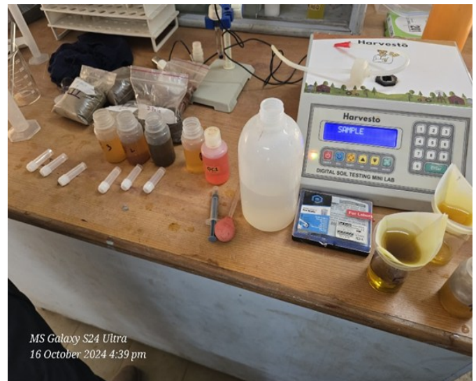
Fig. 1. Laboratory setup for calculating the values of pH and electrical conductivity.
