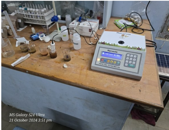
Fig. 2. Harvest soil testing kit setup for electrical conductivity.
