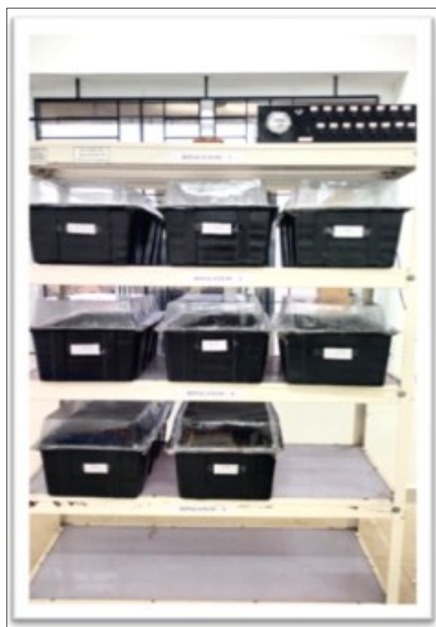
Fig. 2. Container setup to measure the real-time \text{CO}_2 %.
