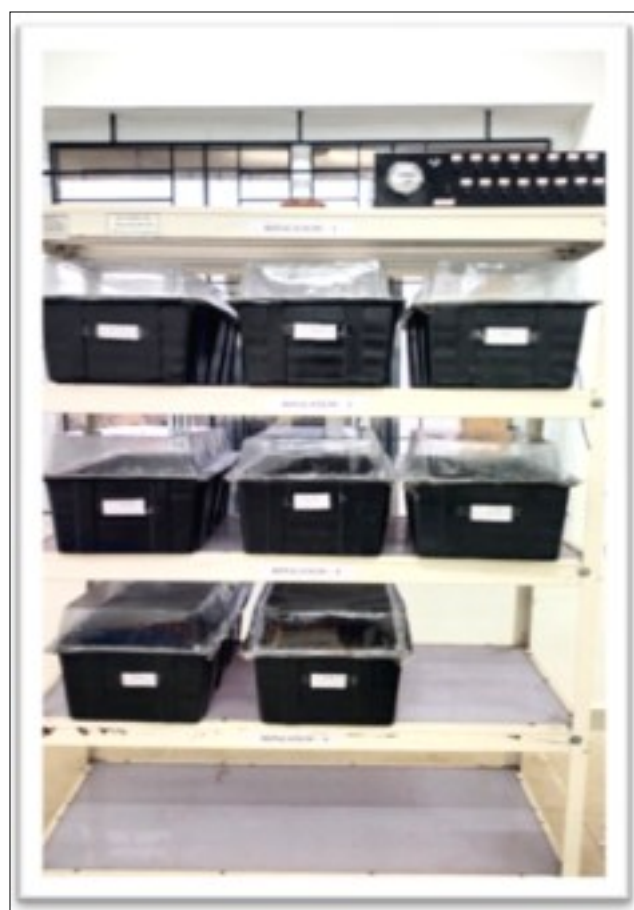
Fig. 2. Container setup to measure the real-time \text{CO}_2 %.
