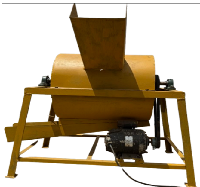
Fig. 1. Front and rear view of the paddy thresher.
