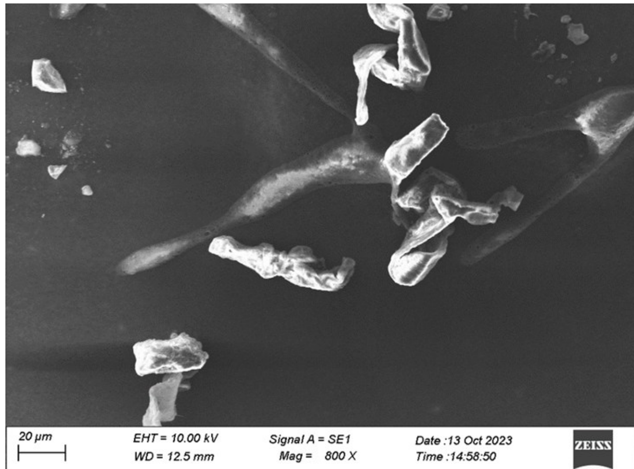
Fig. 4. SEM showing broken fibrils, microstructures, or debris of spirulina ice cream with 800X magnification, 20 μm scale.
