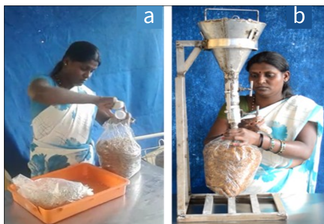
Fig. 1. Manual and spawn spreading machine inoculation: a. Inoculation of mushroom spawn manually, b. Inoculation of mushroom spawn by a spawn spreading machine.
