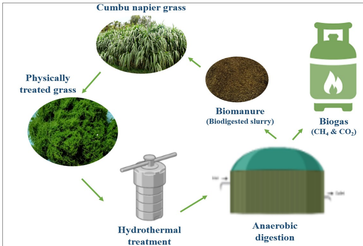
Fig. 1. Process flow diagram of hydrothermal pretreatment of Cumbu Napier grass with cow dung for biogas production.
