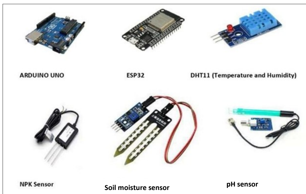
Fig. 5. Internet of things (IoT) sensors used for collecting soil and environmental parameters.
