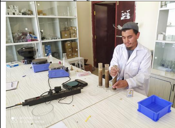
Making soil solution for test the soil texture
