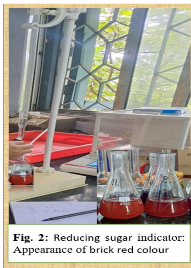
Fig. 2. Estimation of reducing sugars in banana fruit juice showing the development of a brick-red colour reaction.
