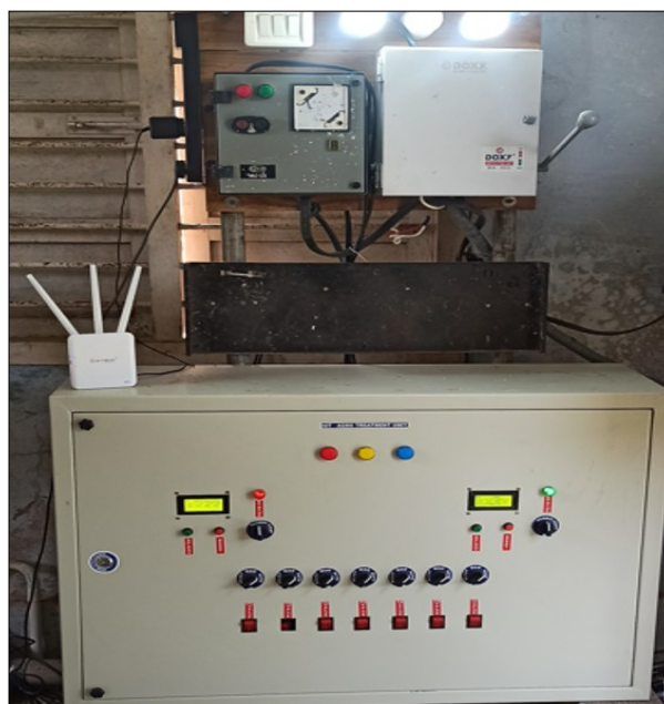
Fig. 2. Internet of things (IoT) based smart irrigation unit.
