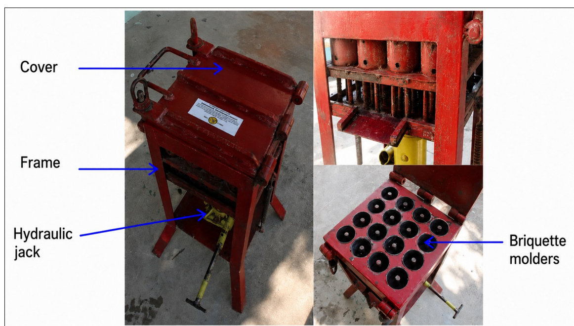
Fig. 2. The hydraulic jack-driven briquetting machine utilised in the briquette production test.
