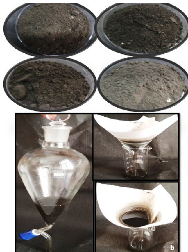
Fig. 1. Photograph showing contaminated soil samples (bagru); (a) Soil samples collection; (b) Solid-liquid extraction.
