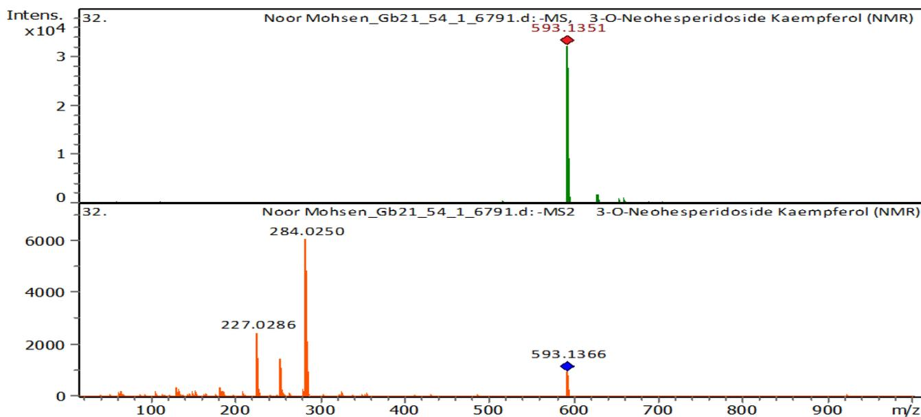
Fig. 4. The mass spectrum of 3-O-Neohesperidoside Kaempferol.
