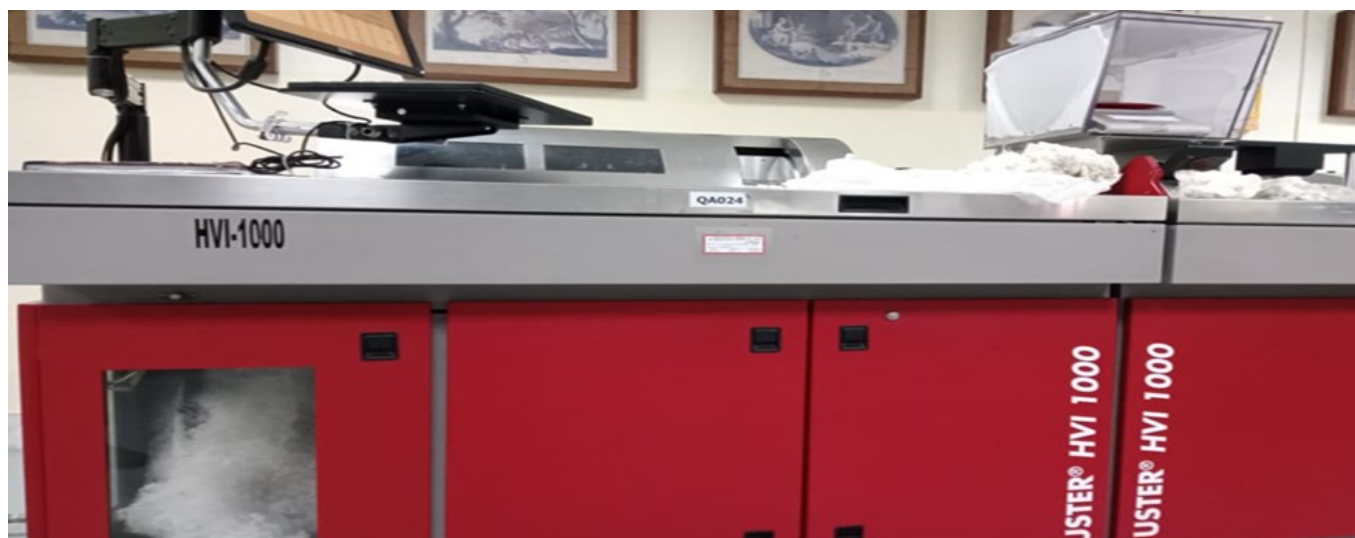
Fig. 2. Uster HVI Fiber testing machine for staple length.
