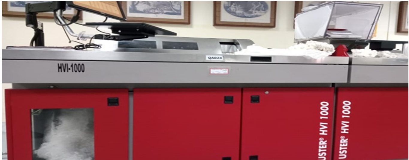
Fig. 2. Uster HVI Fiber testing machine for staple length.
