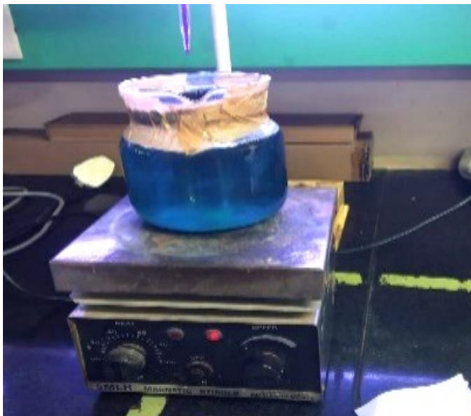
Fig. 4. Shaking and titration against N/10 \text{KMnO}_4 up to golden yellow colour.
