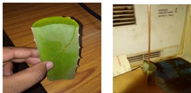
Fig. 1a & b. Sample of Aloe vera leaf cut across cross-section to expose gel material.
