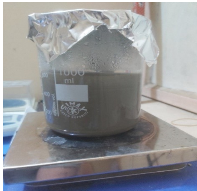
Fig. 1. Extraction of Ammi Majus with solvent by heating and stirring.
