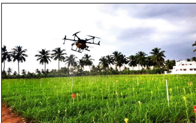
Fig. 6. Foliar application of nutrient spray through drone in the research field.
