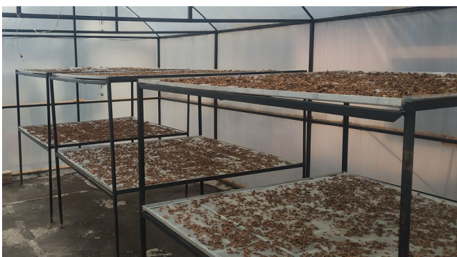
Fig. 8. Dried turmeric inside the tunnel dryer (cumulative time: 97:03 h, day: 5 th , inside temperature: 32.6°C, inside humidity: 50.6%, outside temperature: 22.5°C, outside humidity: 58.6%, sunshine intensity: 255 W).
