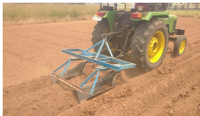
Fig. 3. Furrow irrigated raised bed former.
