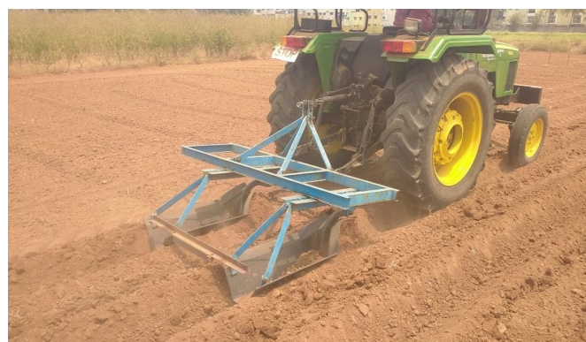
Fig. 3. Furrow irrigated raised bed former.
