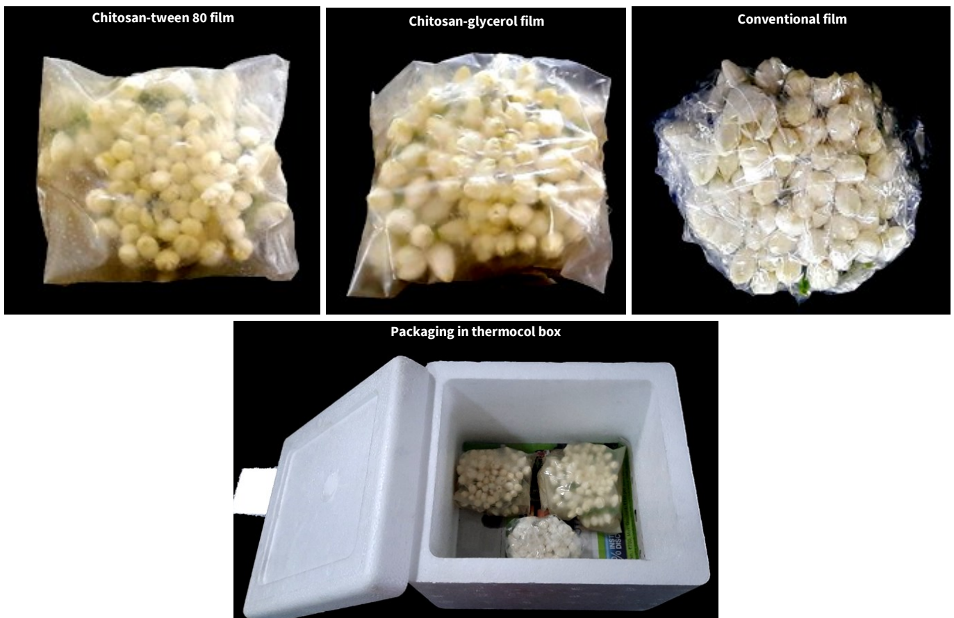
Fig. 2. Packaging of jasmine flowers in chitosan-based films, conventional film and placed in thermocol box for storage under refrigeration.
