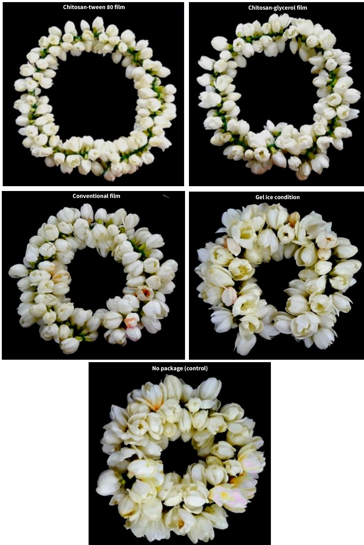
Fig. 6. Results show the quality of jasmine flowers packaged in chitosan-based films, conventional film, gel-ice condition and with no packaging after 3 days (72 h) of storage under refrigeration at 5°C.
