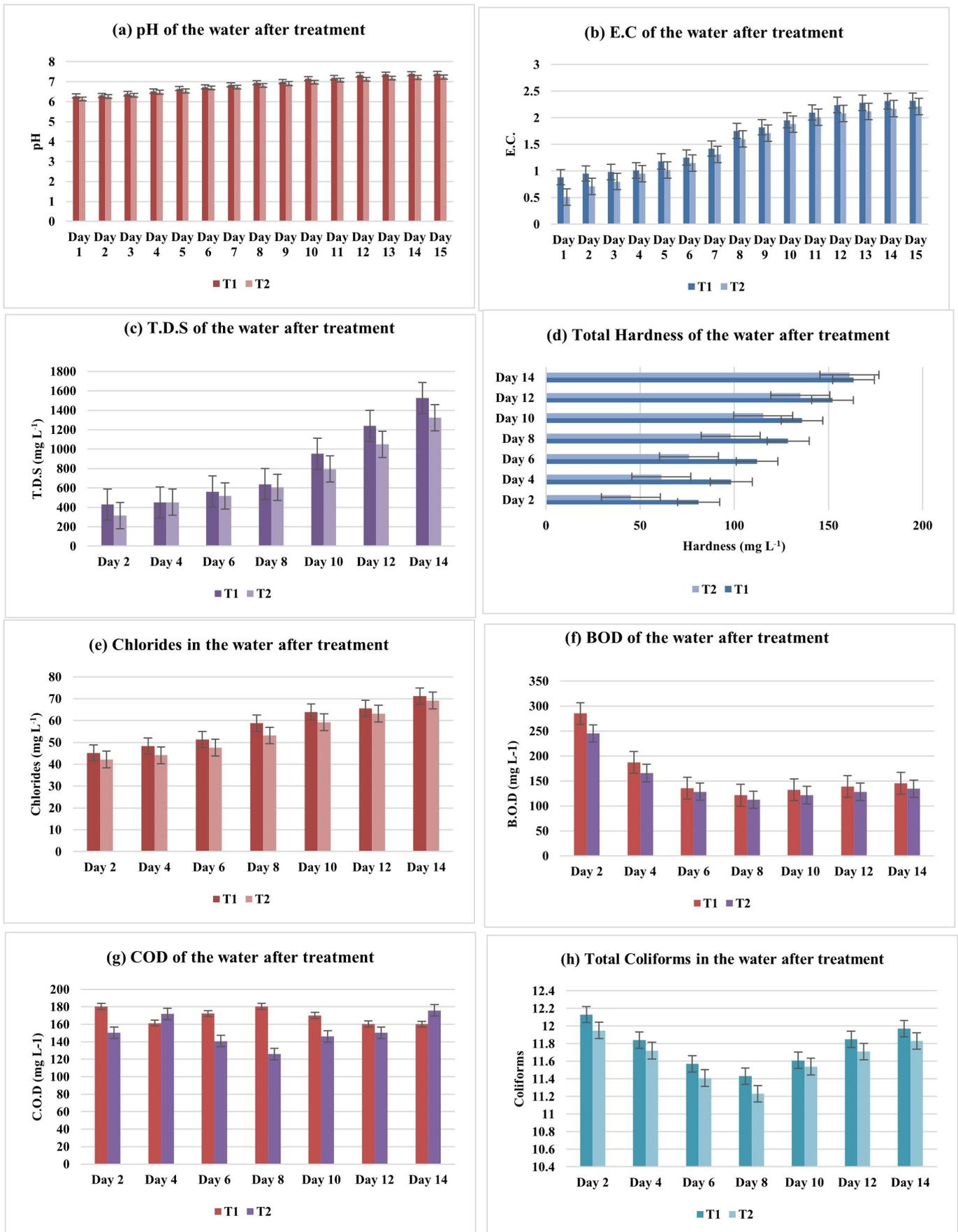
**Fig. 5.** Graphical illustrations represent the reduction of efficiency of the columns showing the variation in (a) pH, (b) E.C., (c) TDS, (d) Hardness, (e) Chlorides, (f) BOD, (g) COD and (h) Coliforms.
