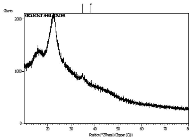
**Fig. 4.** XRD pattern of groundnut shell nanosheet.
