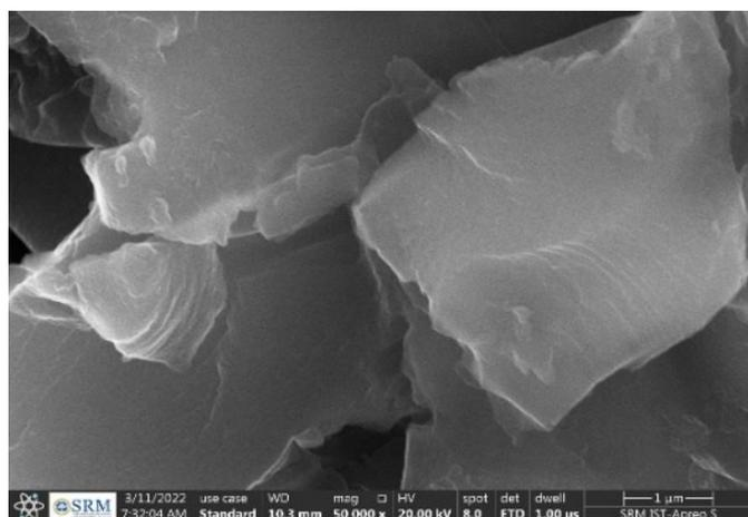
**Fig. 3.** SEM (1µm) micrographs of groundnut shell nanosheet.
