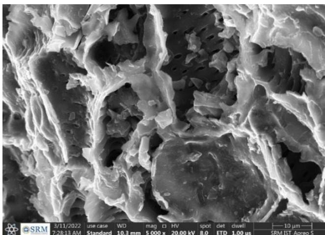
**Fig. 2.** SEM (10µm) micrographs of groundnut shell carbon mixed with KOH.
