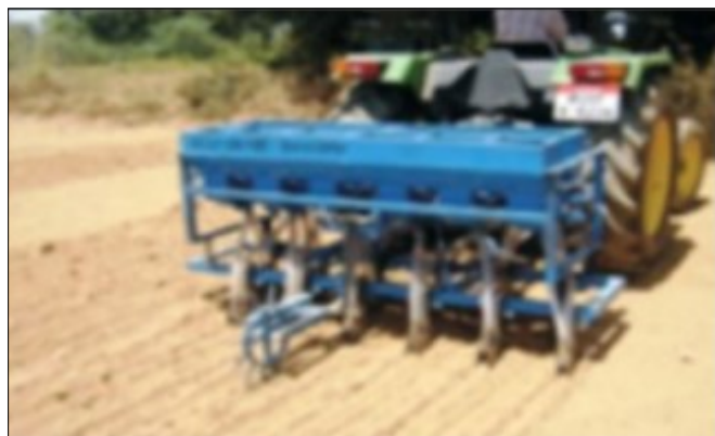
Fig. 4. Tractor mounted garlic planter (a) 12-row planter (22) (b) 9-row planter (24).
