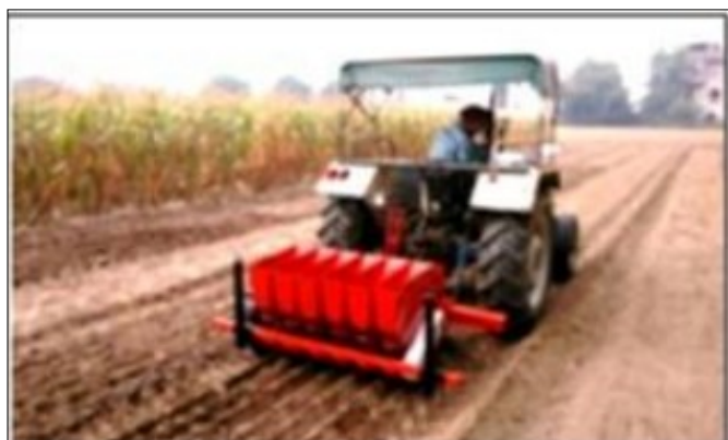
Fig. 5. Tractor operated garlic planter (a) 6-row planter (Mehta, 2015) (b) Tractor operated garlic planter (Zilpilwar et al., 2019).
