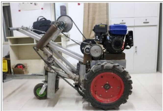
Fig. 9. Self-propelled Garlic Harvester (Sun et al. 2018).
