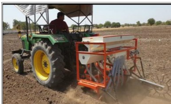
Fig. 5. Tractor operated garlic planter (a) 6-row planter (Mehta, 2015) (b) Tractor operated garlic planter (Zilpilwar et al., 2019).
