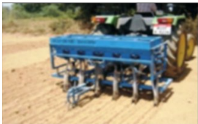
Fig. 4. Tractor mounted garlic planter (a) 12-row planter (Singh, 2010) (b) 9-rows planter, IARI Annual Report, 2014.
