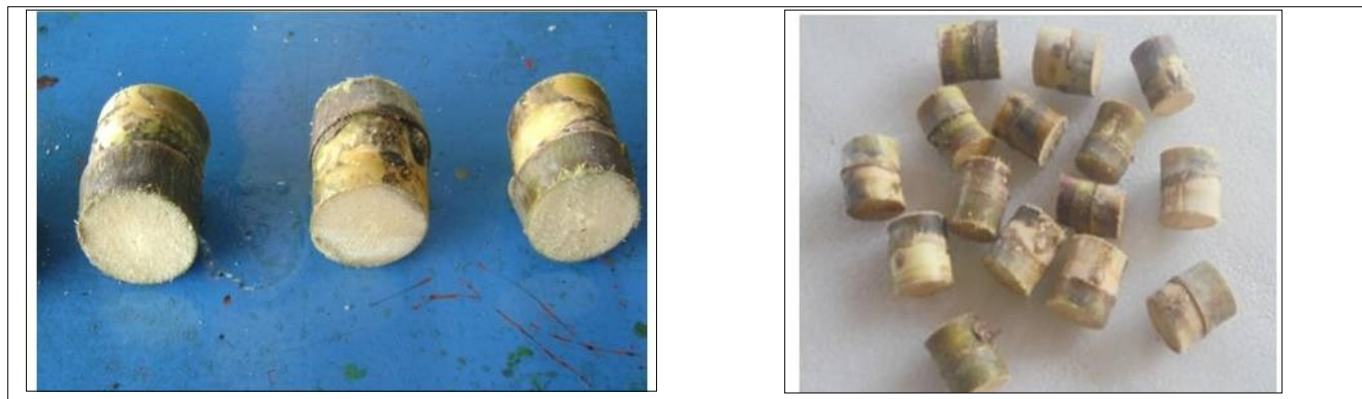
Fig. 5. 35 mm length single bud sugarcane setts at 2200 rpm with 200 mm diameter of cutting blade.
