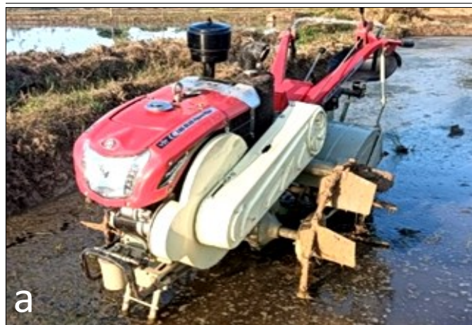
Fig. 1. The prime movers used for the puddling operation. (a) 16 hp power tiller; (b) 13 hp power tiller.
