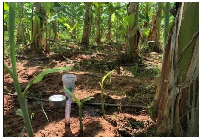
Fig. 2. Tensiometer installation at the experimental field.
