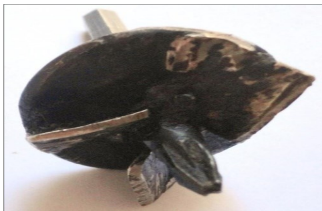
Fig. 2. Newly designed disc with three radiating blades and pointed projection.
