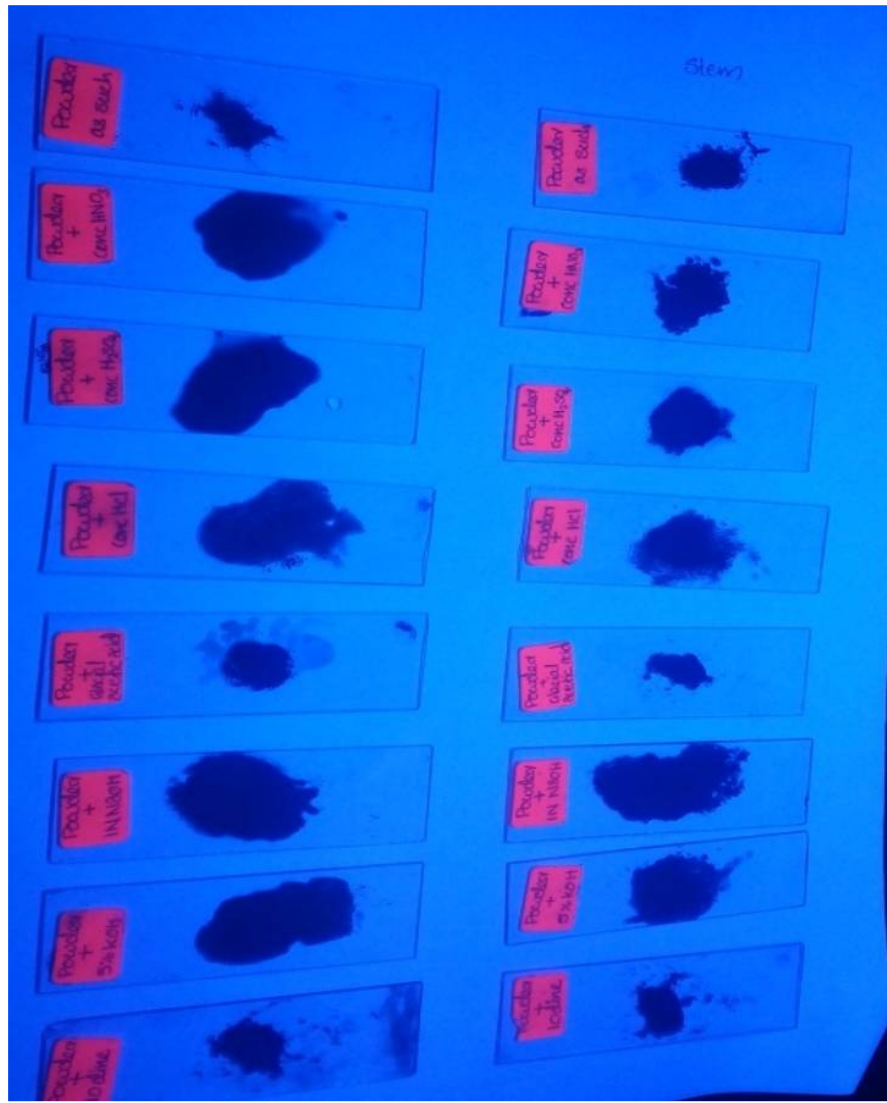
Fig. 3. Absence of fluorescence in all samples of Phyllanthus spp. when kept under UV Transilluminator.
