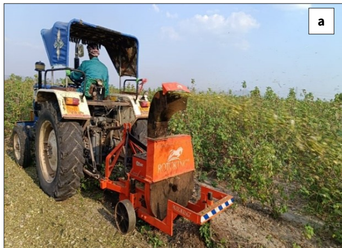
Fig. 11. a. In-situ incorporation of stubbles through shredder in cotton; b. In-situ incorporation of stubbles through shredder in castor.
