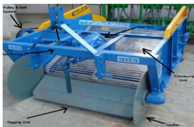
Fig. 7. Tractor drawn root crop harvester for potato and ginger crop (58).
