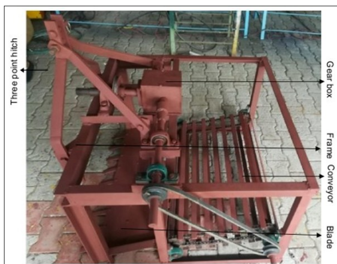
Fig. 6. Mini tractor operated turmeric harvester (55).
