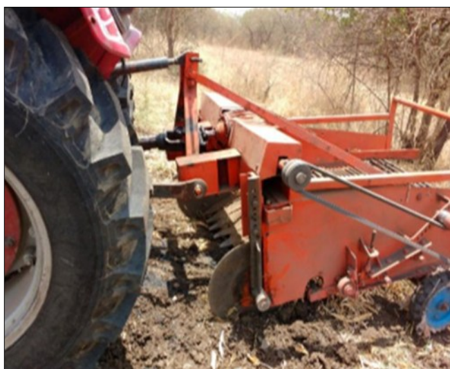
Fig. 5. Tractor PTO-operated turmeric digger-cum-separator in field (38).
