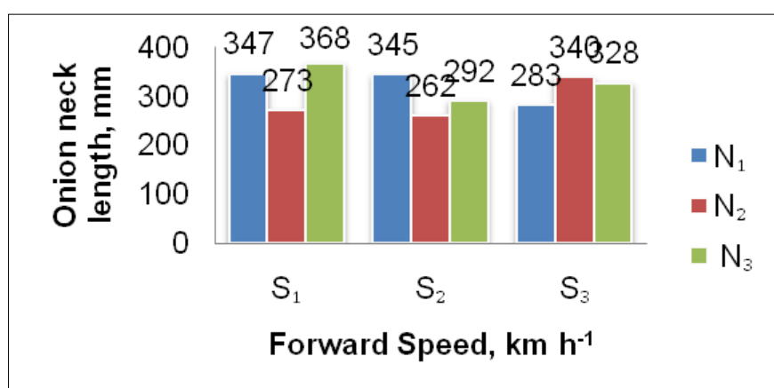
Fig. 11. Effect of forward speed (km h -1 ) and peripheral speed (m s -1 ) on onion neck length with flat type string and two cutting strings
