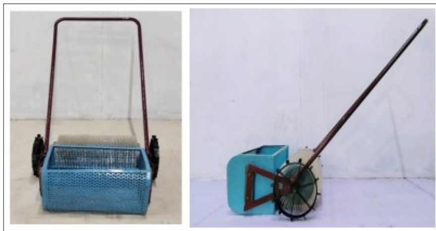
Fig. 7. Mechanical neem fruit picker cum collector (62).
