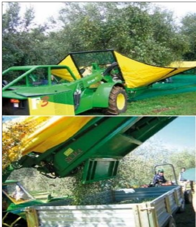
Fig. 5. Mechanical harvesting of olives with a trunk shaker with a reversed umbrella interceptor (32).
