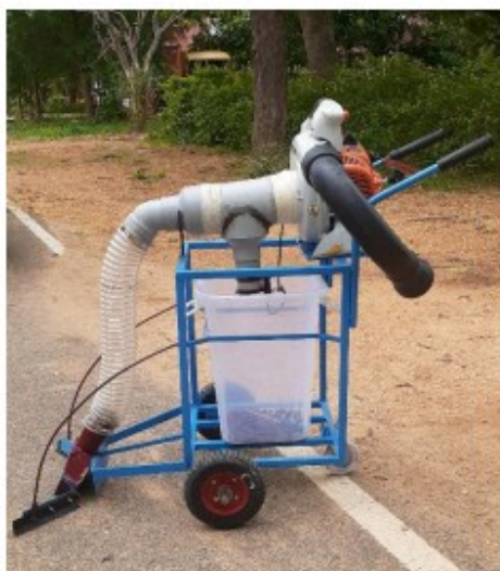
Fig. 6. Pneumatic suction type ground collection system (16).
