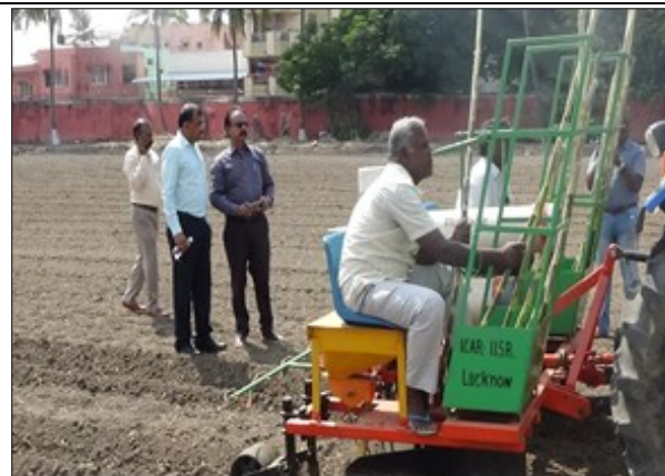
Fig. 1b. Field operation of tractor operated deep furrow sugarcane sett cutter planter.
