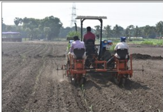
Fig. 1a. Field operation of tractor operated sugarcane settling transplanter.
